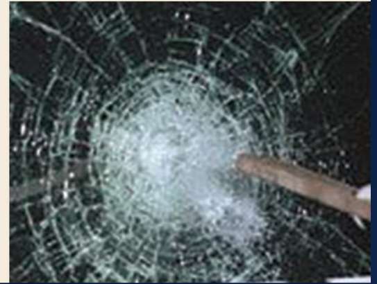
9 LB 2X4 MISSILE SHOT AT 50 FT/SEC TESTS IMPACT WINDOW
