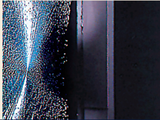
LAMINATED GLASS MAY CRACK UNDER PRESSURE, BUT TENDS TO REMAIN INTEGRAL, ADHERING TO THE PLASTIC VINYL INTERLAYER
