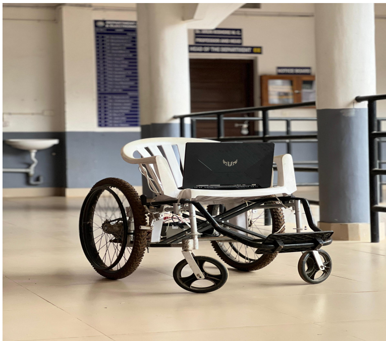
Fig 22: Front view of eye ball controlled wheelchair
