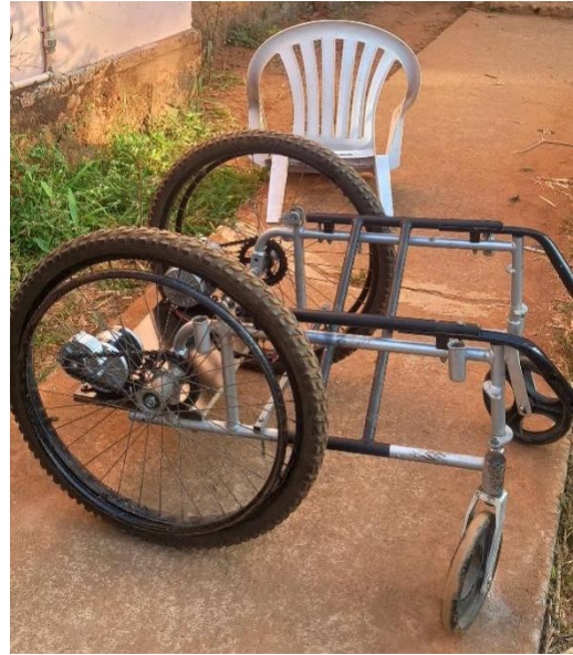
fig 14.2: connecting motor & sprocket
