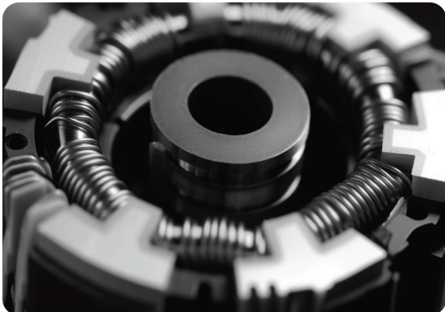
The core and windings of a traditional motor
