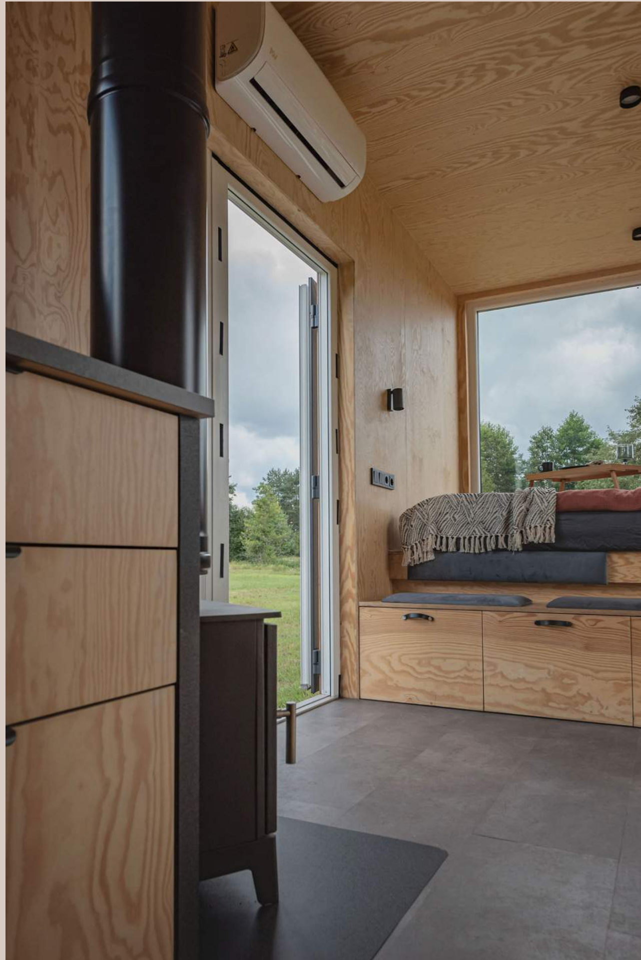
EXAMPLE OF INTERIOR – FLOORS: VINYL, A/C, WOOD STOVE, INSULATED CHIMNEY, STORAGE UNDER THE BED
