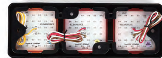
环氧灌封 Epoxy sealed
