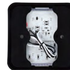
环氧灌封 Epoxy sealed
