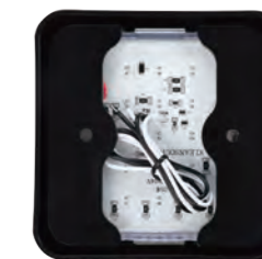
环氧灌封 Epoxy sealed
