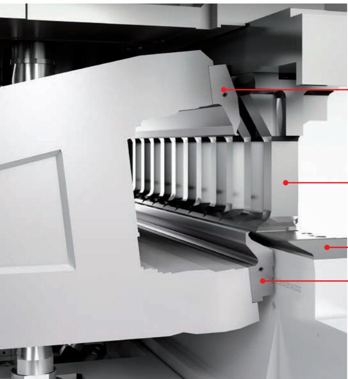
**A** The upper and lower blades (A, D) are the two tools featuring interpolated controlled movement and responsible for bending.
