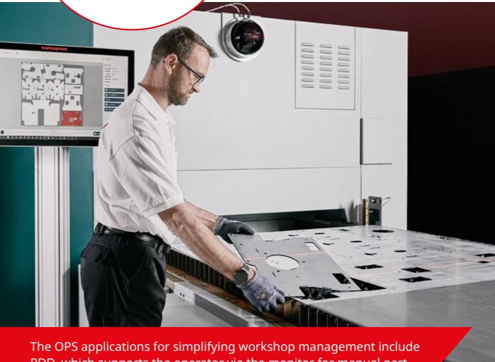
The OPS applications for simplifying workshop management include PDD, which supports the operator via the monitor for manual part separation and sorting, and LPG, which laser-guides the operator in the pick-up sequence.
