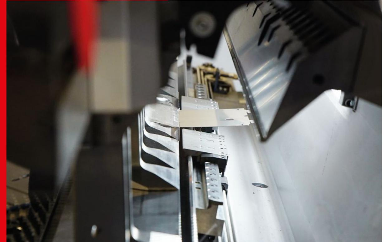
To automate some of its bending activities, Metalsystem chose a P2-2120. It is an extremely versatile solution, used to bend panels up to 2180 mm, with a maximum bending height of 203 mm. The panel bender also has a DPM – an optional gripping device coupled to the manipulator which is used to bend panels that have internal windows or are below the minimum bending size – and a special P tool, which further extend the field of application.
