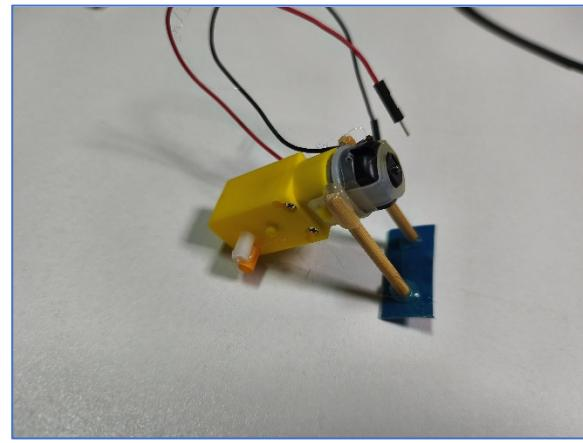
**Step 8 – Add the Red Walking Arms:** Connect the legs to the robot body by inserting the small wood sticks to the straw joints of the motor body.
