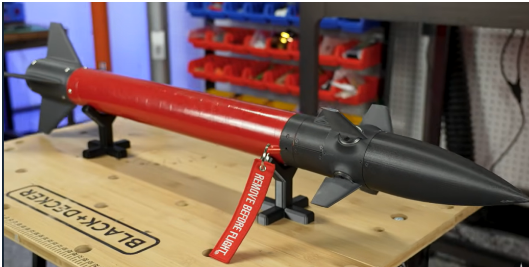
Figure 1. Model rocket using forward canards for roll control, showing private implementation. Screenshot from Project Horizon [3].
