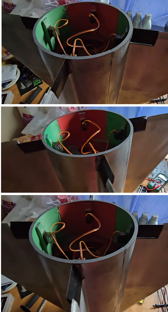
Figure 13. Fin-can prototype used for bench-level roll-control demonstration. The silver cylindrical body was manually rotated to show the black control surfaces responding in the opposing direction.
