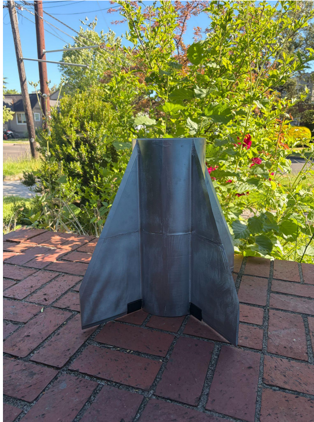
Figure 15. Fully integrated fin-can
