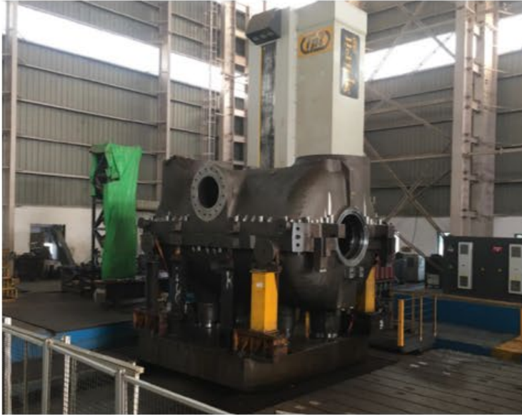
CNC Horizontal Boring Machine X – 22m Y – 7m Z – 2m , W – 1m Indexing Table – 4.5m x 4.5m Weight Capacity – 120 tons Universal Head Facing & Turning Head
