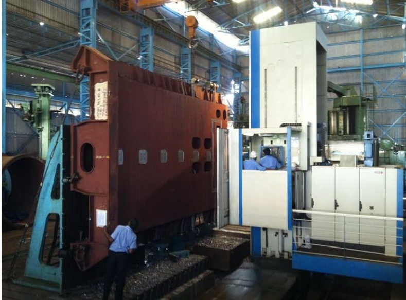
CNC Horizontal Boring Machine-1 X – 10m Y – 4.5m Z – 1.5m , W – 0.7m Indexing Table – 2.5m x 3m Weight Capacity – 35 tons Universal Head Facing & Turning Head
