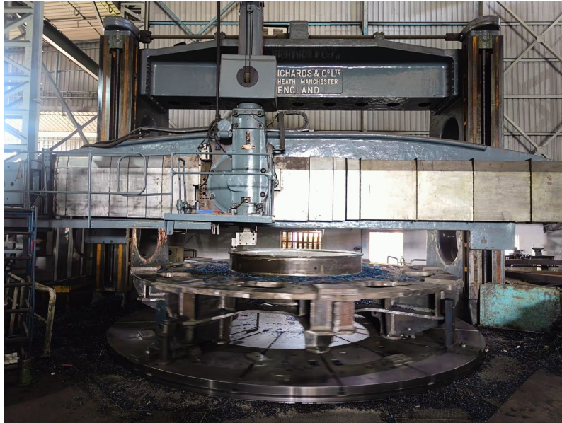
CNC Vertical Lathe (VTL)-1 Table Dia – 6.3m Max Swing – 6.9m Max Working Height – 3.7m Tool Travel – 2.5m Weight Capacity – 100 tons Grinding Attachment
