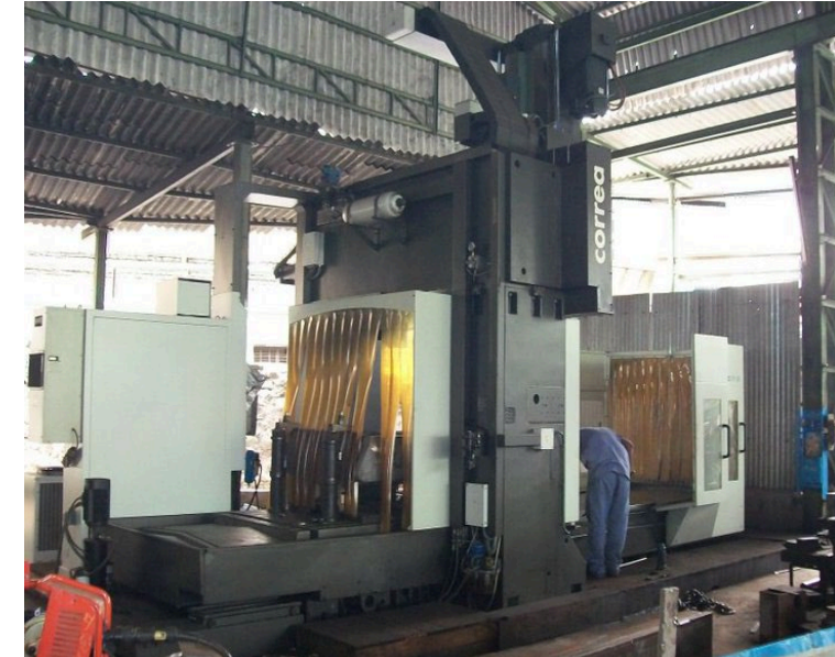
CNC Vertical Machining Center X – 2.5m Y – 1.7m Z – 1.2m Max Height – 1.5m Weight Capacity – 15 tons Universal Head Facing & Turning Head
