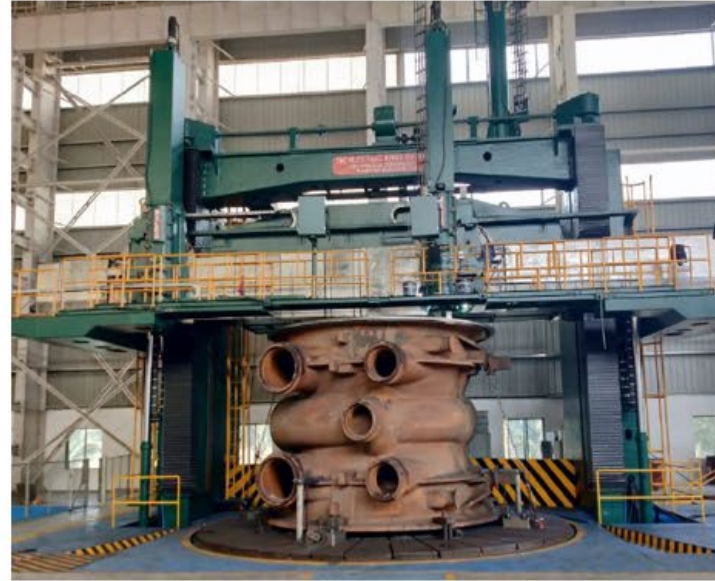
CNC Vertical Lathe (VTL) Table Dia – 7.6m Max Swing – 9.2m Max Working Height – 5.1m Tool Travel – 3.5m Weight Capacity – 250 tons Grinding Attachment
