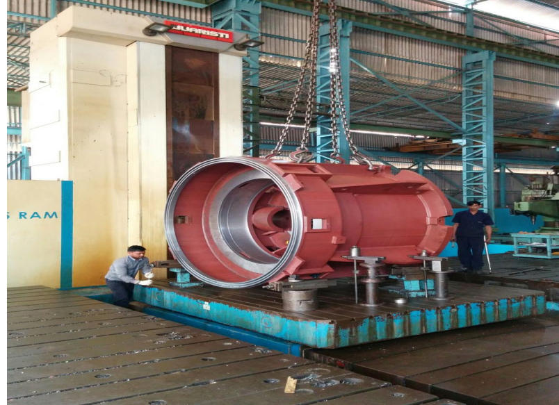
CNC Horizontal Boring Machine-2 X – 10m Y – 4m Z – 1.2m , W – 0.8m Indexing Table – 3.5m x 3m Weight Capacity – 70 tons Universal Head Facing & Turning Head
