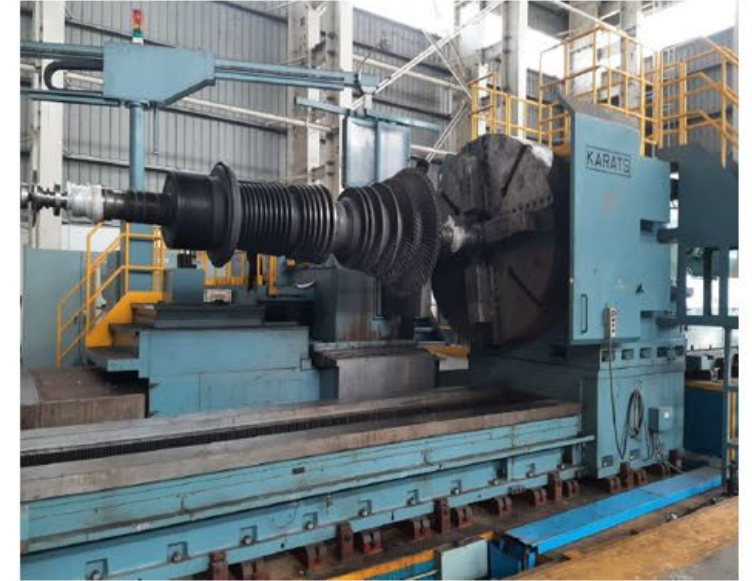
CNC Horizontal Lathe Chuck Dia – 2.1m Max Swing – 3m Max turning Length – 12.25m Weight Capacity – 110 tons Grinding Attachment Various Stead Rests
