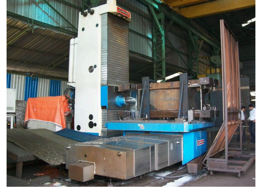
CNC Horizontal Boring Machine-3 X – 4m Y – 3m Z – 1.5m , W – 0.7m Indexing Table – 2.5m x 3m Weight Capacity – 25 tons Universal Head Facing & Turning Head
