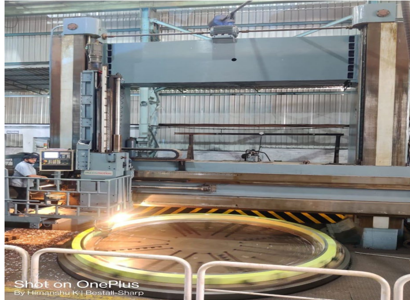
CNC Vertical Lathe (VTL)-2 Table Dia – 4.6m Max Swing – 5.2m Max Working Height – 4.7m Tool Travel – 2.5m Weight Capacity – 70 tons Grinding Attachment
