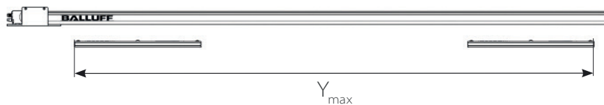
Fig. 2.2-4. Minimum and maximum distance between adjacent interval markers
