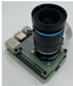
Figure 4.1: Raspberry Pi 4 module with an HQ camera attachment on a specific case which eases mounting of the set-up.
