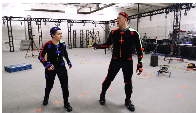
Figure 1.1: Example of Motion Capture in Animation, at the House of Moves studio. This system has 72 infrared cameras surrounding the capture space and each performer has to wear a special suit with numerous reflectors [1].
