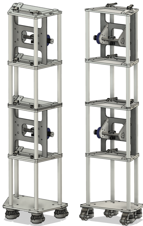
Figure 3.7: Front & Back view of the system's CAD. This example is composed of the base compartment, two sensor compartments and an empty compartment for height adjustment.
