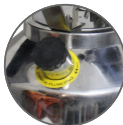
Chemical Filling Space
