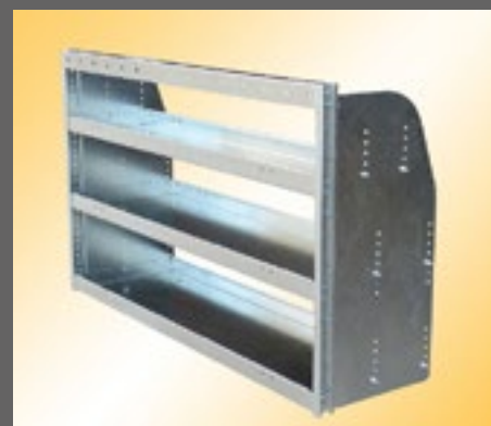
UTE RACKING Assembly required. P/N: EL-RA1663-00 RACK SIZE OD: W1060 x H630mm x D350 KIT HAS 3 SHELVES - SIZES (ID) Top shelf ID: W1020 x D230mm (1x narrow top shelf) 2nd & 3rd ID: W1020 x D300mm (2x full width shelves) Universal fitting kit included.
