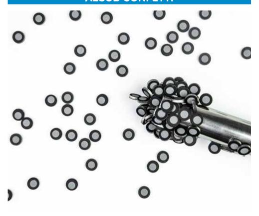
AESUB Confetti is a time-saving and efficient solution for 3D scanning that adds a touch of fun to the process! These metallic dot-coins feature reference points on both sides, making them perfect for scanning complex areas, like car interiors. Simply toss them onto the surface — such as a dashboard or other interior parts —
