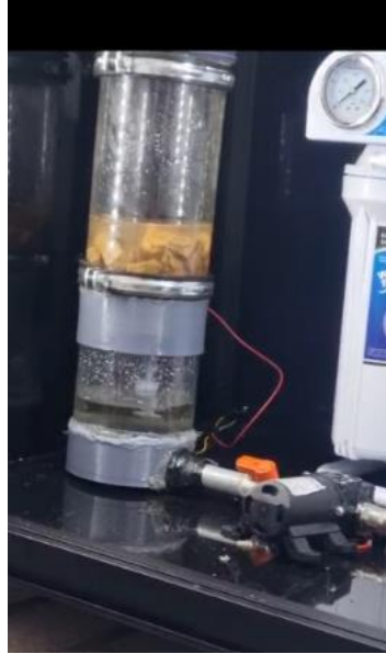
Figure 13: Muddy water before and after gravity filter.
