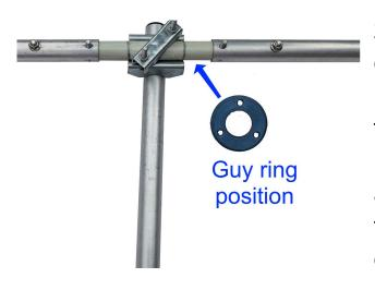
2. Fit the main elements onto the ends of the GRP rod and align the bolt holes. Note: now is the time to fit the guy ring if required. Insert the 2 outermost 35mm bolts and tighten the serrated nuts. The top main element section (with the end hat securing bolt) is on the right in the picture.
