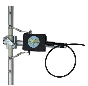
7. Your co-axial cable can now be fitted to the matching transformer with a PL259 connector. Seal the connector against moisture using the self amalgamating tape. Wrap the tape tightly from the socket to the plug. Form a small stress relief loop prior to taping the coax cable to the centre support arm using PVC insulating tape.
