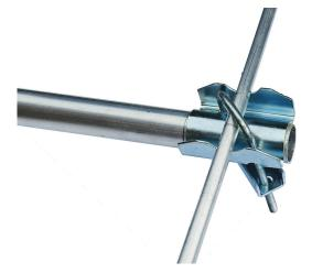
5. Attach the lower capacity hat element to the bottom of the lower main element using the second cross clamp as shown. Centralise the capacity hat element using the alignment marks and ensure it is parallel to the top element before tightening the clamp bolts. Fit the plastic end caps.
