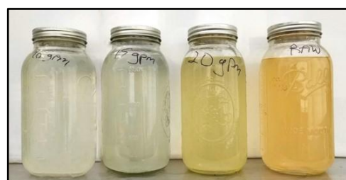
PRODUCED WATER BEFORE AND AFTER TURBOCOAG® PROCESSING.
