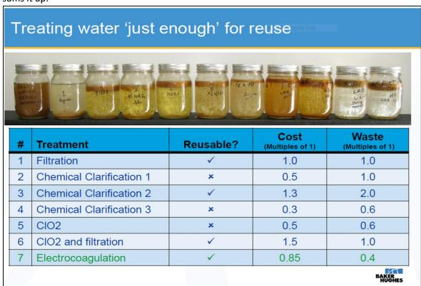
This slide was captured from a Baker Hughes website which discussed the advantages of EC vs chemicals, outlining potential cost advantages, and large waste disposal advantages. What it does not point out is that EC is also a **biocide** due to OH- radicals produced at the cathode.
