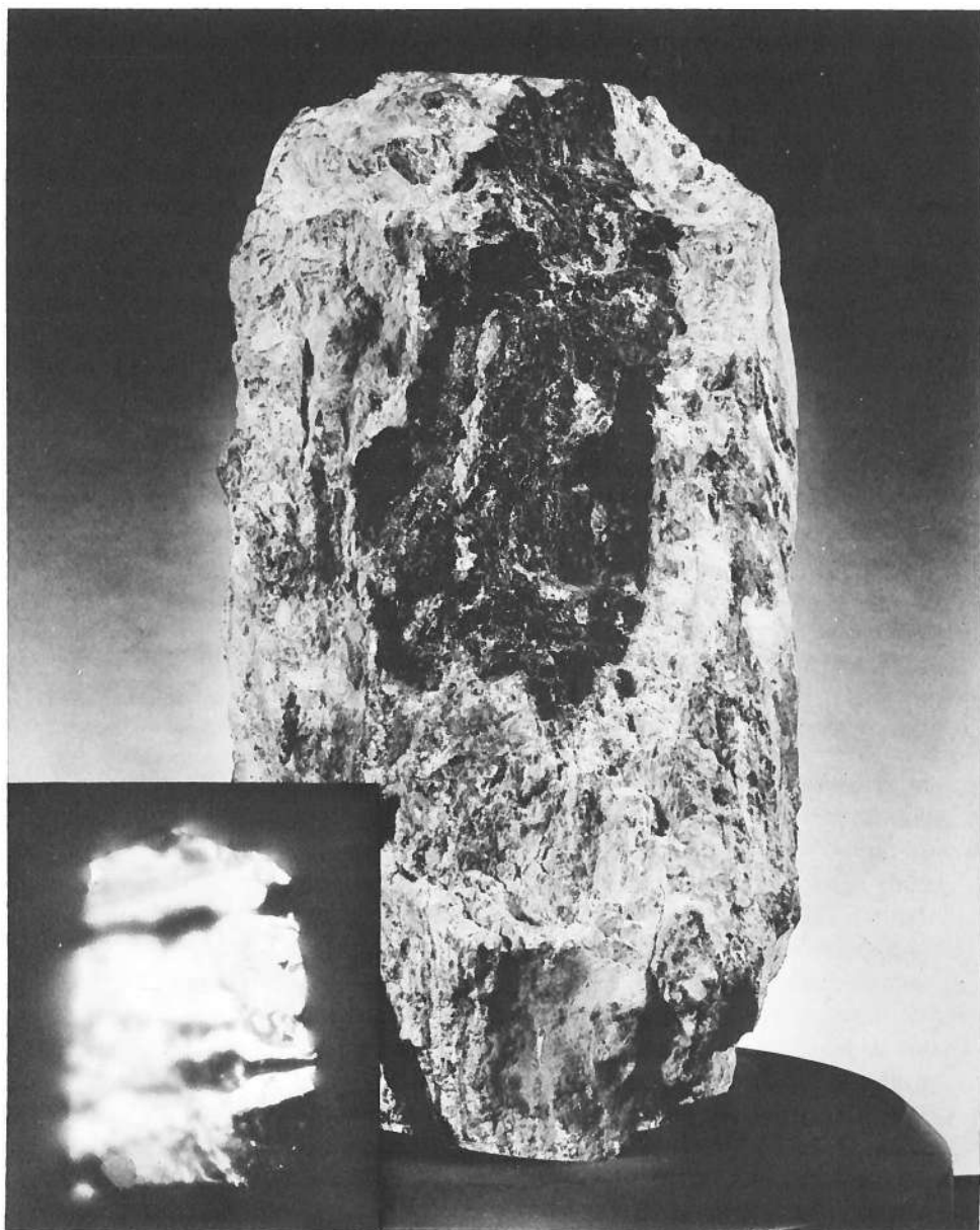
Uranium ore. The black portion is pitchblende (uranium oxide); the inset in the lower left corner is an autoradiograph produced by pitchblende's radioactivity.
