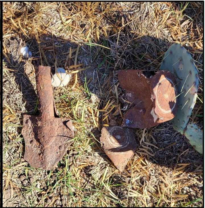
Severely heat-deformed shovel and solder top cans
