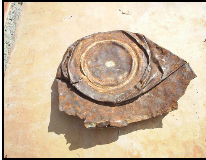
Lead-soldered lap side seam No.2 can
