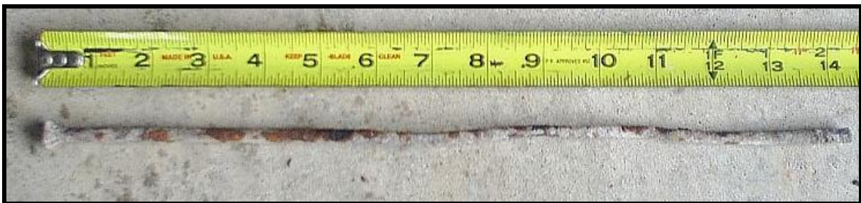
14-inch threaded bolt for box buggy seat
