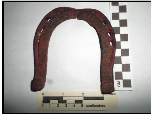
Hand-forged Spanish Mule shoe with crack and heavy wear
