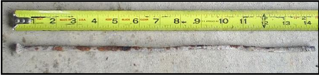
14-inch threaded bolt for box buggy seat
