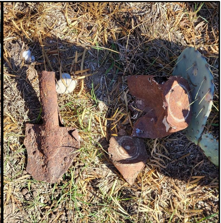
Severely heat-deformed shovel and solder top cans
