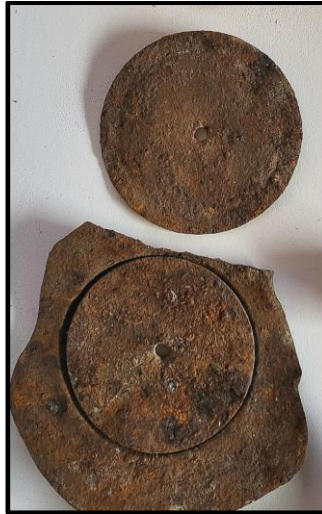
Hole-in-Cap Can Lids missing lead solder
