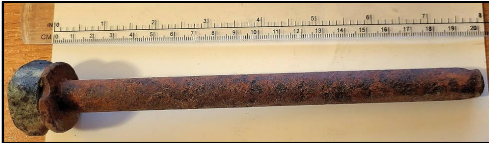
Broken Heavy Picket Pin
