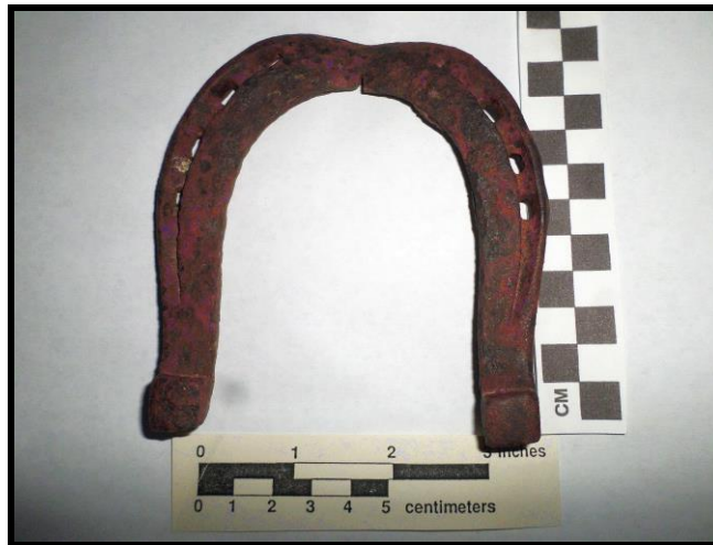
Figure 18: Hand-forged mule shoe with crack and heavy wear
