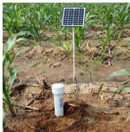
Figure 2: Example of a soil moisture sensor installation in an agricultural field
