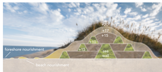
Figure 6. Construction principle and heights (m) of the new dune
