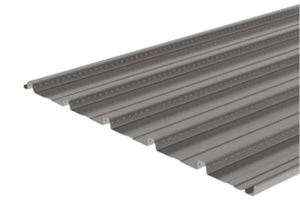
Ares23 offers a sustainable decking solution, meticulously designed with high tensile steel to ensure a minimum yield stress of 500 MPa. It comes in various base metal thicknesses, including 0.75mm and 1.00mm. The galvanized coating, Z275, maintains a minimum of 275g/m2, meeting the AS1397:2001 standard. Additional thicknesses and coating options are available upon request, based on availability.
