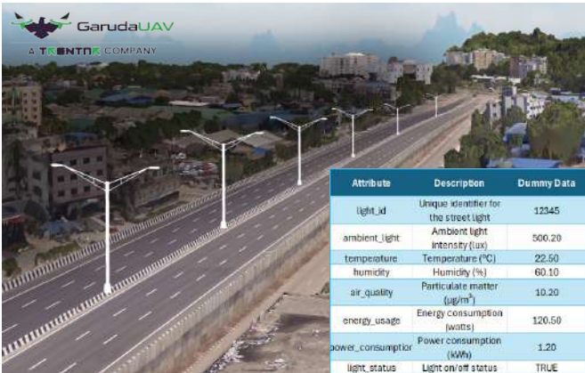
Figure 3: Vector models of streetlights integrated into the 3D texture model to demonstrate the potential final appearance of the infrastructure. The attribute table highlights potential data that could be collected from IoT devices on these streetlights. Source: GarudaUAV.
