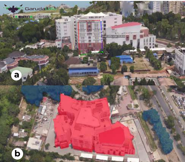
Figure 2: (a) Height and length data of a building extracted from a 3D texture model, allowing for enhanced visualization of spatial relationships and scale; (b) The buildings (in red) and trees (in blue) are digitized to create a 3D vector model from the 3D texture model.
