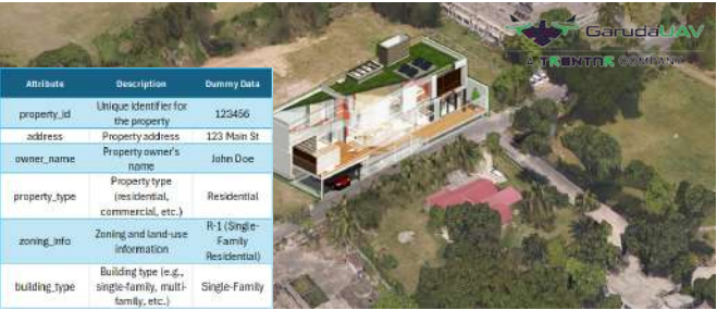
Figure 4: BIM model of a house integrated with 3D texture data, showcasing a realistic visualization of the final appearance. The attribute table highlights the land record information that can be digitally stored and regularly updated through real-time data integration.
