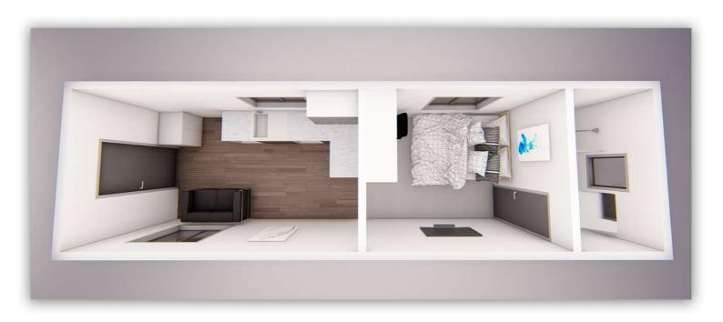
This is a 9m long by 2.6m wide Living modular unit which is a portable structure.
