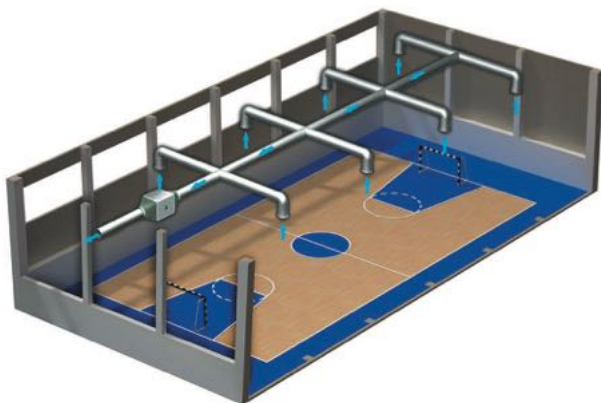
VS fan gym ventilation example
