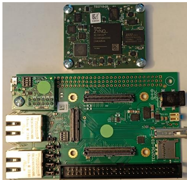
Figure 2-9. Low-cost FPGA board for building the clock demonstrator.
