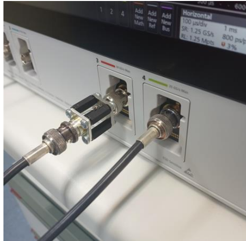
Figure 6-15. Galvanic insulation mounted in a support to BNC connectors at the Oscilloscope input 3 of one of the signals from the Evaluation Board.
