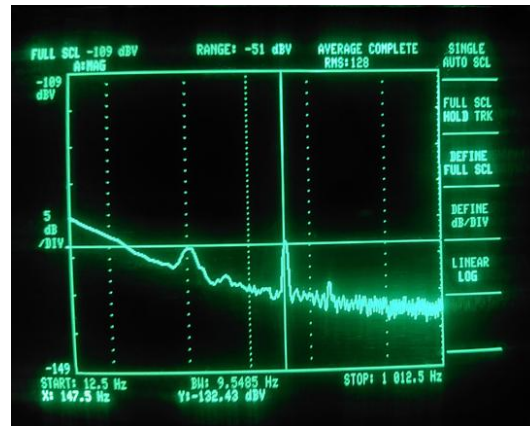
Figure 12 Noise spectrum for a 6 V lead-acid battery
