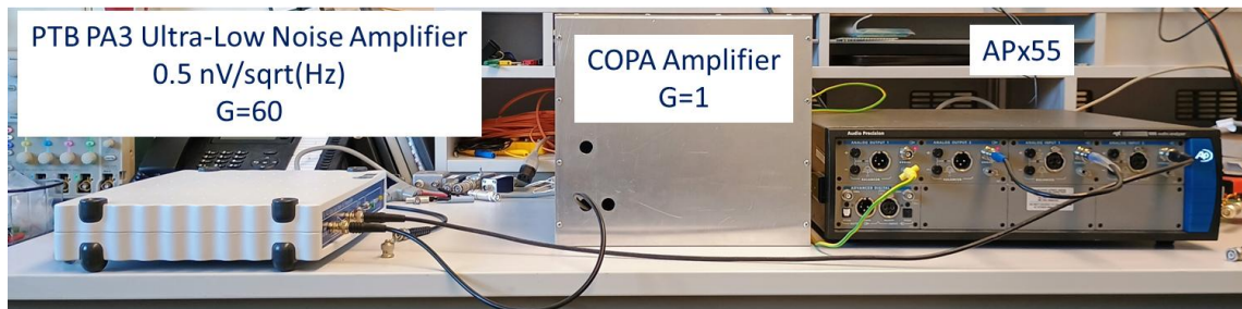
Figure 16: Noise measurement setup, using the PTB PA3 Ultra-low noise amplifier to amplify the noise from the COPA to be detected by the APx555
