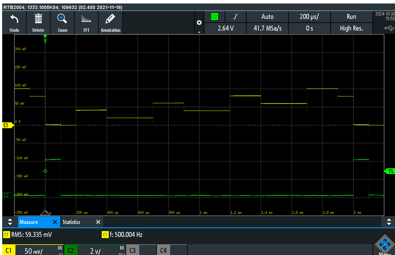
Figure 7-5: Integrator with TMUX1133, 4 cycles
