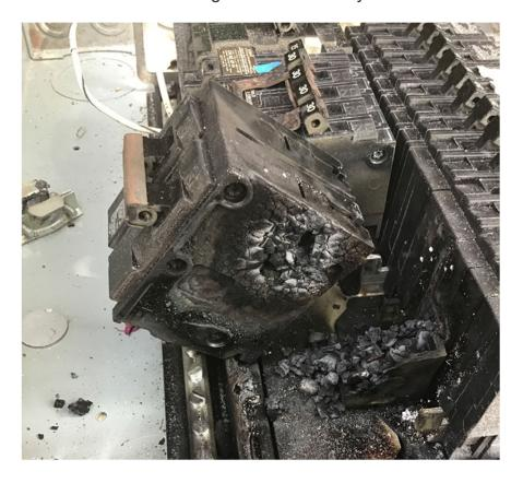
Unfortunately, this breaker failure happens every year in homes equipped with Federal Pacific Electric (FPE) Stab-Lok panels. Despite this information and the number of electricians and home inspectors who warn against this equipment, FPE Stab-Lok panels were never officially recalled.
