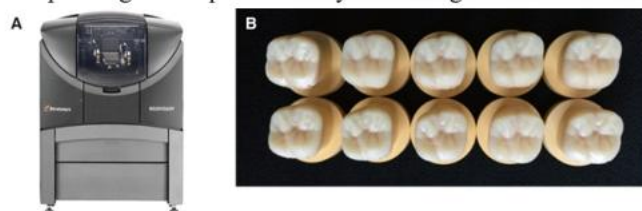
Figure 3. (A) 3D printing system (Stratasys), (B) Manufactured crown
