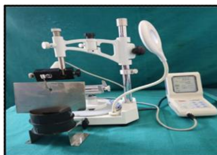
Fig: Endomotor secured to a Surveyor during Procedure
