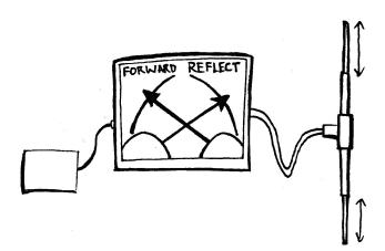
attach the antenna to the end of a mast piece 10 feet long. The element to which the braid or shield of the coax is attached must be pointing down Support the mast so that it stands straight up with the antenna at the top. It is best to do this outside.
