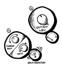
applied and the output level. Set the ratio control to the infinity setting; this enables hard limit function. Attack and decay can be set around mid position. Adjust the threshold and the input level until the gain reduction shows activity. Adjust the output level so that the indicator lights or meters show a 0 dB output level.
