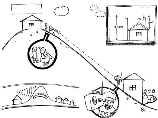
It is good practice to keep the transmitter some distance from the audio studio since the radio frequency emissions from the transmitter can get into the audio equipment. causing noise and hum. Your transmitter should be set up in another room, attic space, etc. as close to the antenna as possible. Keep the distance transmitter from the antenna as short as possible. This will minimize signal loss in the coaxial cable feeding the antenna.
