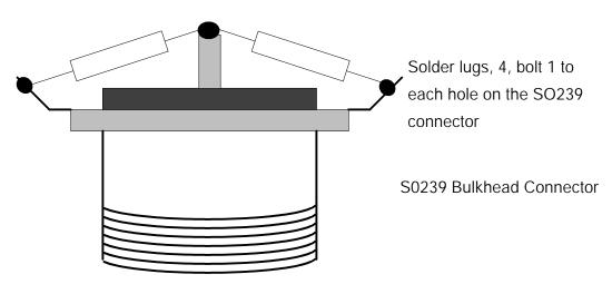
Use a mating connector, a dual male PL259 (Radio Shack #278-192 or equivalent) to connect this directly to the transmitter output S0239
