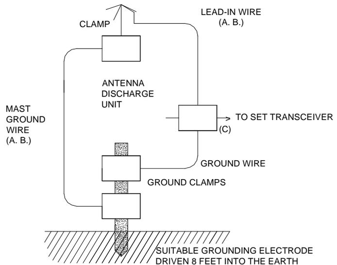
C – Mount antenna discharge unit as possible to where the lead-in wire enters the house.
