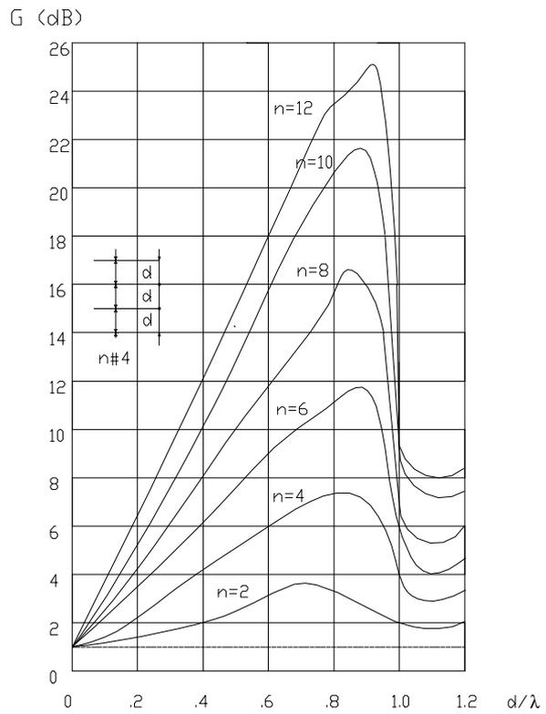
Gains diagram of horizontal dipole
