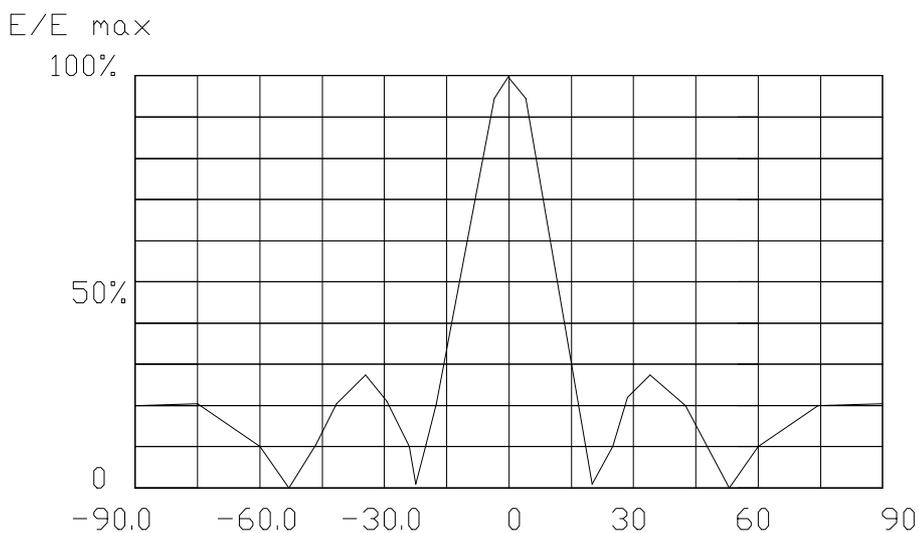
Vertical radiation pattern of a curtain composed of elements with a space of  $0.5\lambda$ . between each other and feeder with the same current and phase.
