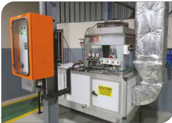
Life size equipment to train the skills needed for the setting of system controls and safety devices.
