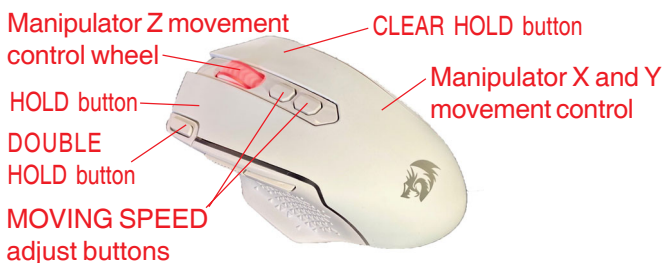
Wireless Mouse for left side (Holding) control
