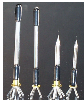
Unpulled and Pulled 7, 4-barrel Pipettes
