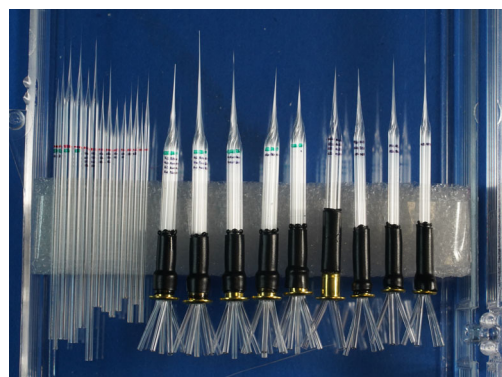
Pulled single, 3, 4, 7-barrel pipette samples from all preset sequences with each shipped out unit
