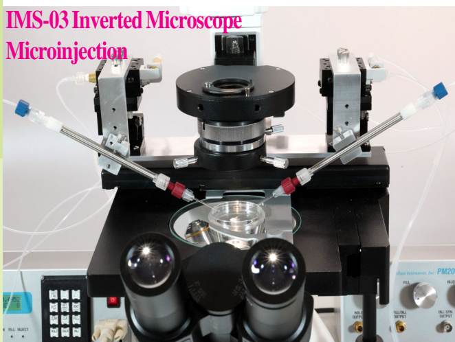
Mouse Control Micromanipulators and Microinjection Work Station
