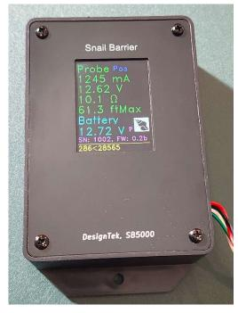
the controller in a system that also needs a power supply typically a battery, solar panel, and solar charge controller along with an under-water probe typically made from two stainless steel bands. This controller has several features:
