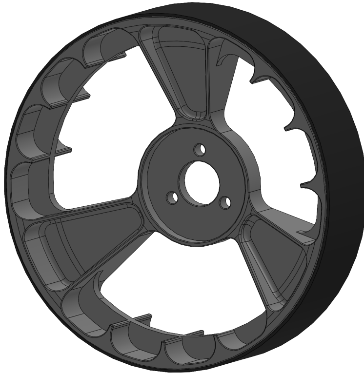
Figure 21: Isometric view of the wheel design. The tire is affixed to the wheel via first sewing a flat sheet into a hoop, using stainless steel lockwire for thread, and then pressing it over the wheel center. A knurled surface over the outer diameter of the wheel center ensures good retention of the tire.
