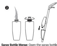
**Spray Bottle Merge:** Open the spray bottle, fill with water→tighten the cap→screw into the bottom of the connecting tube!
