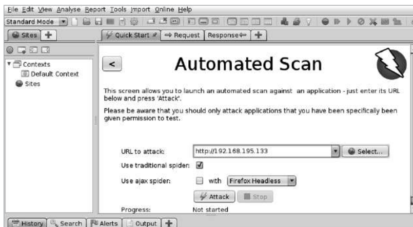
Figure 6-18: An automated scan set up to scan a target with OWASP ZAP
