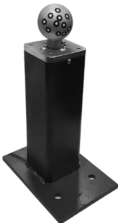
Fig. 8. The custom-built, GOM marked spinning device used to assess the GOM spin rate calculations.
