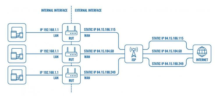
The example above depicts a scenario where the Internet Service Provider (ISP) provides different routers with IP addresses that are unique and constant (they never change for each device). In this case the router performs the NATing process instead of the ISP, thefore the ISP is "transparent" when the router sends or receives data from remote hosts on the internet.
