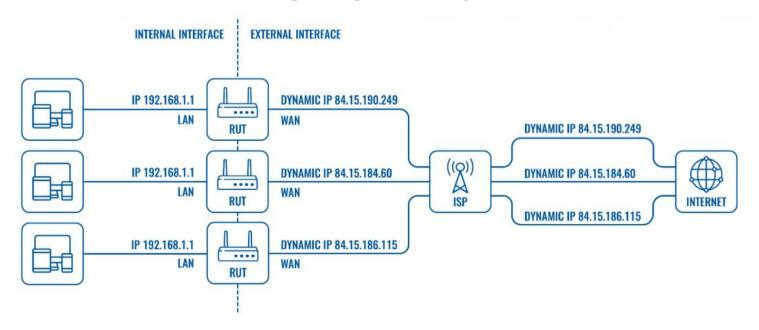
From the example above we can see that in case of dynamic IP addresses the ISP provides the routers with private WAN IP addresses that are then "translated" into public IP addresses when connecting to
