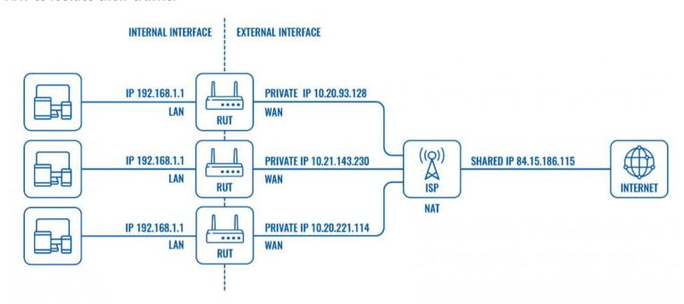
In the example above we can see that it is possible for multiple devices (even websites) to share a single public IP address. An ISP provides clients with private WAN IP addresses and then uses NAT to differentiate to which host specific data packets should be directed to.
